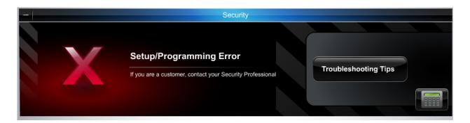
Error 1000 is caused the lack of PSD (Panel Security Data) being sent from the Panel to the Total Connect 2.0 system. There are a few causes of this ranging from no initial PSD received to the Panel or Alarmnet Device programming.
